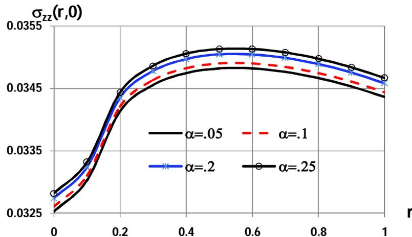
Fig. 2 Effect of graded parameter  $\alpha$  of indenter on  $\sigma_{zz}(r,0)$
