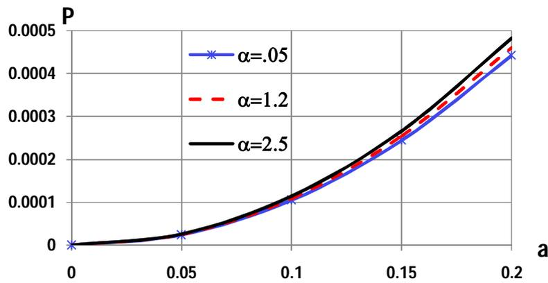
Fig. 6 Effect of graded parameter  $\alpha$  on applied load P
