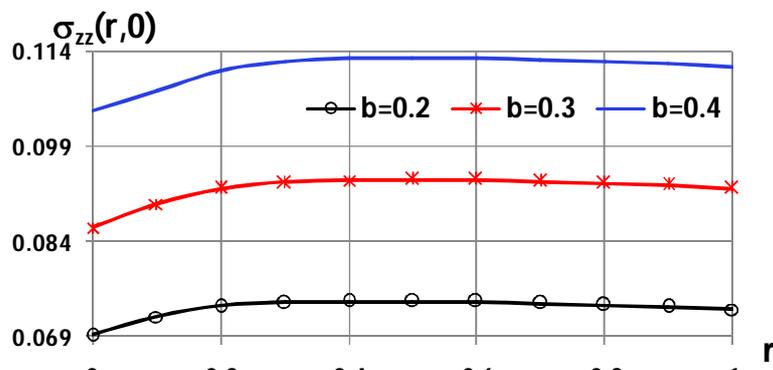
Fig. 4 Effect of radius of the flat end of the indenter on  $\sigma_{zz}(r,0)$
