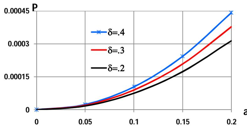
Fig. 7 Effect of indentation depth  $\delta$  on applied load P
