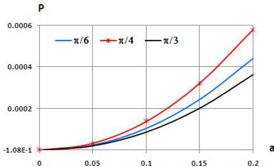
Fig 9 Effect of semi vertical angle  $\Phi$  of indenter on applied load  $P$
