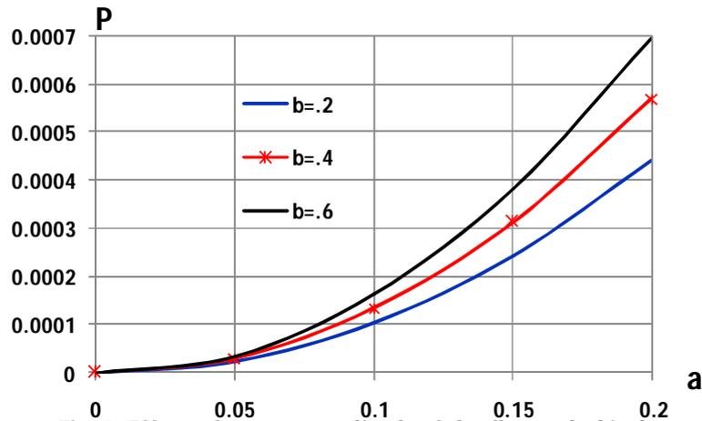
Fig. 8 Effect of contact radius  $b$  of the flat ended indenter on applied load  $P$
