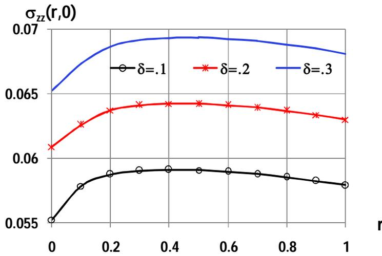
Fig. 5 Effect of indentation depth  $\delta$  of indenter on  $\sigma_{zz}(r,0)$
