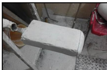
**Figure (2):** Gypsum mold
