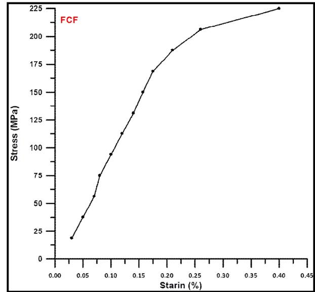
**Figure (9):** Stress-strain curve for stacking sequence (FCF)
