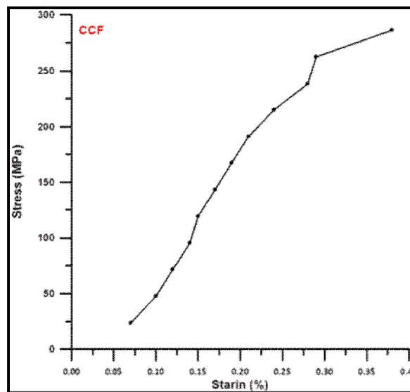
**Figure (6):** Stress-strain curve for stacking sequence (CCF)
