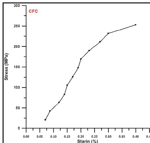
**Figure (7):** Stress-strain curve for stacking sequence (CFC)
