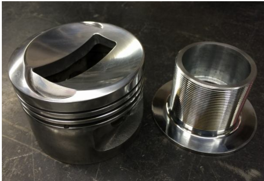
Fig:-3 Split off piston edge of pivot after machining
