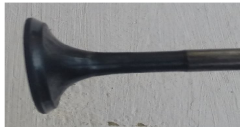
Fig 7: Exhaust Valve: After cleaning
