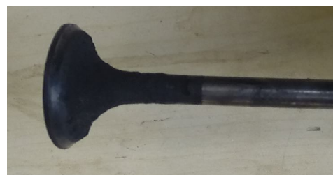
Fig 9: Exhaust Valve: After 10 hours test on fuel mixture
