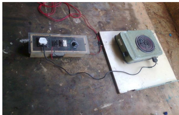
Fig 2: Load given to an engine during running on fuel mixture
