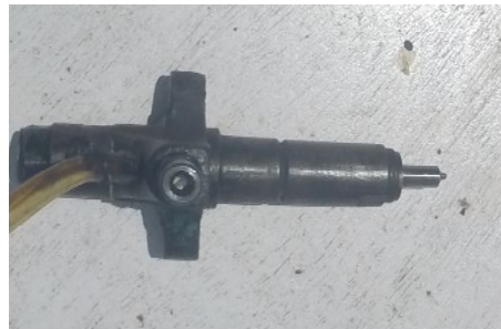
Fig 6: Fuel injector: After cleaning
