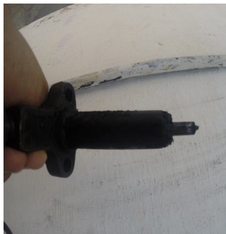
Fig 4: Fuel Injector- With sticky carbon depositions
