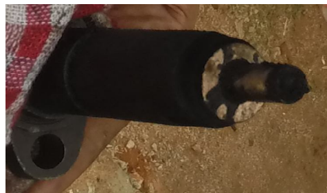
Fig 8: Fuel injector: carbon deposits after 10 hours test on fuel mixture
