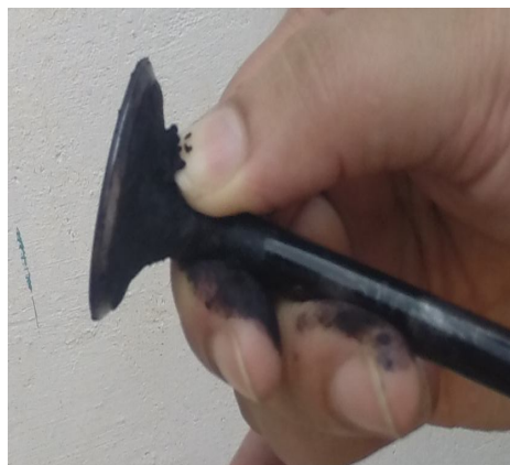
Fig 5: Exhaust valve - With sticky carbon depositions
