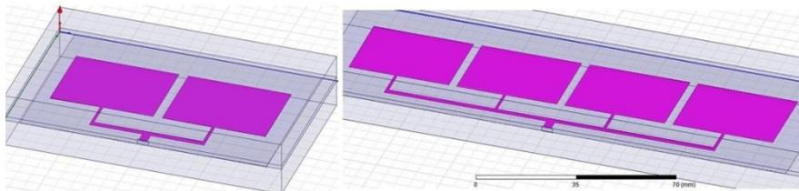
**Figure 2** Two and four elements microstrip patch antenna array
