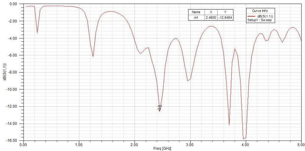
Figure 8 Simulated  $S_{11}$ (dB) on FR4 for quad patch antenna
