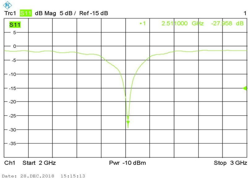
**Figure 5** Experimentally measured  $S_{11}$ (dB) on FR4 for single patch antenna
