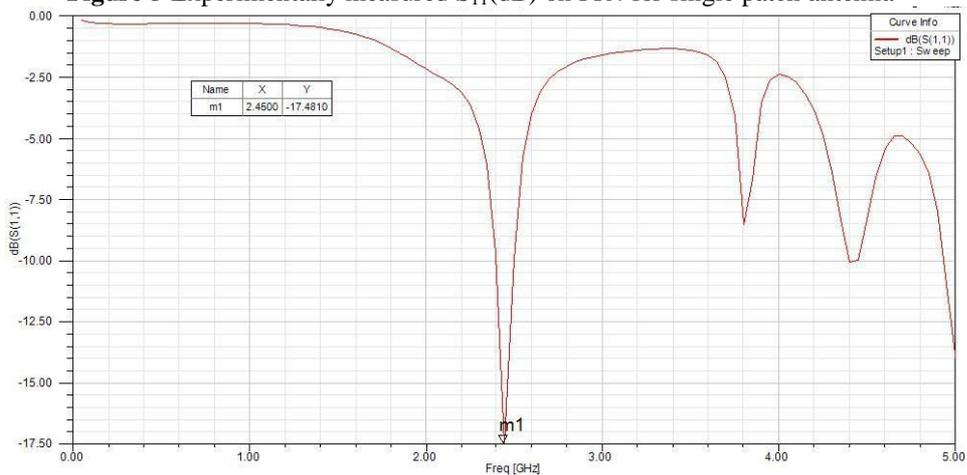
**Figure 6** Simulated  $S_{11}$ (dB) on FR4 for dual patch antenna
