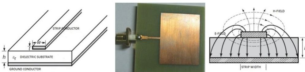
Figure 1 Rectangular microstrip antenna configuration, practical realization and E&H fields
