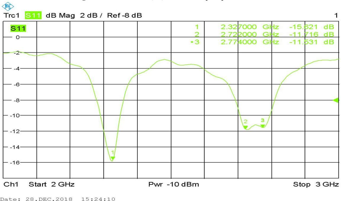
Figure 9 Experimentally measured  $S_{11}$ (dB) on FR4 for dual patch antenna
