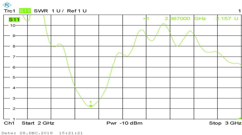
**Figure 7** Experimentally measured  $S_{11}$ (dB) on FR4 for dual patch antenna
