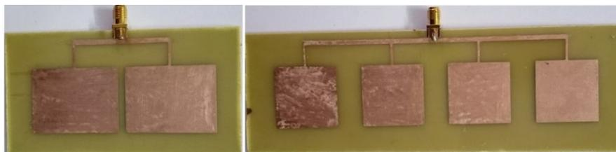
**Figure 3** Fabricated two and four elements microstrip patch antenna array
