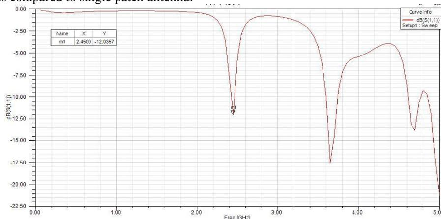
**Figure 4** Simulated  $S_{11}$ (dB) on FR4 for single patch antenna
