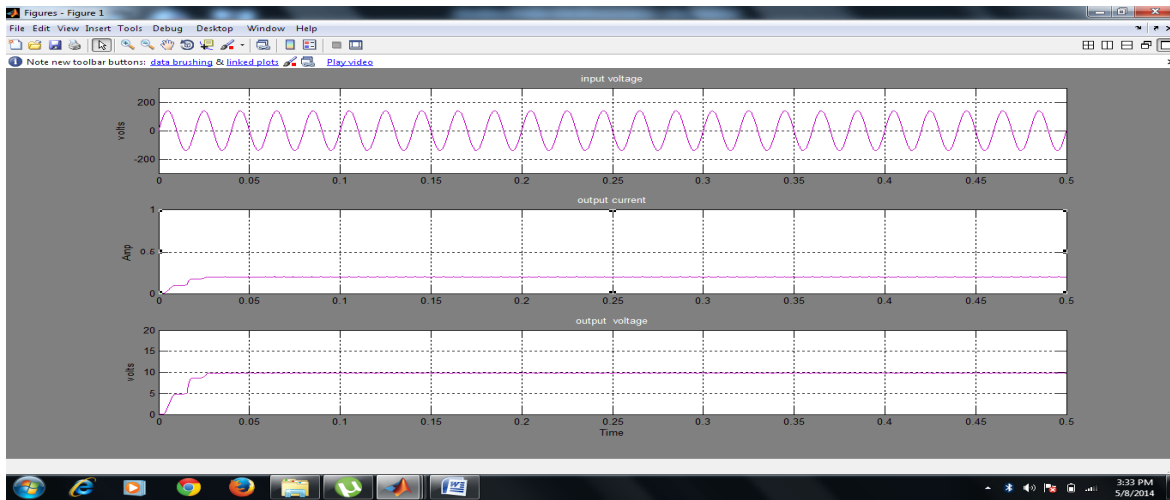
Figure 7. Output Voltage and current with 140 V input voltage at load resistance 50Ω
