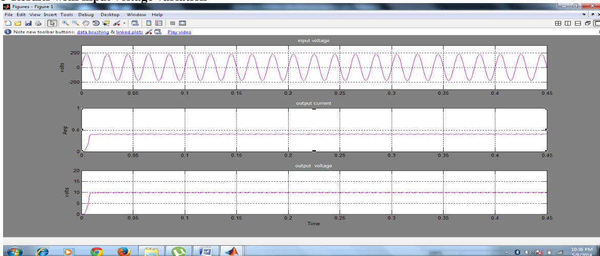
Figure 8. Output Voltage and current with 180 V input voltage at load resistance 25Ω
