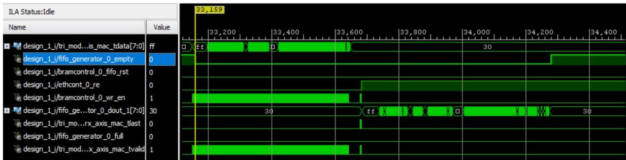
Figure 7 Ethernet Reception and Storing To FIFO Obtained in an ILA
