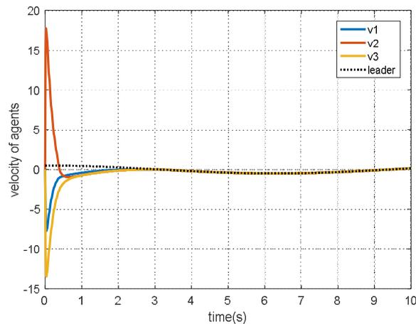
**Figure 5** Consensus tracking results for velocity  $v$  for case 1
