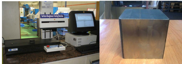
Figure 1. Surface Roughness Tester used for Design of Experiments and preparation of work piece for CNC milling.
