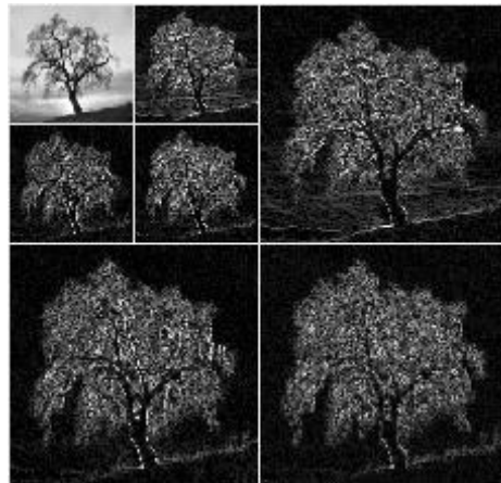
Figure 2 Resulting sub-bands for a 2-level DWT (original image in Figure 1)
