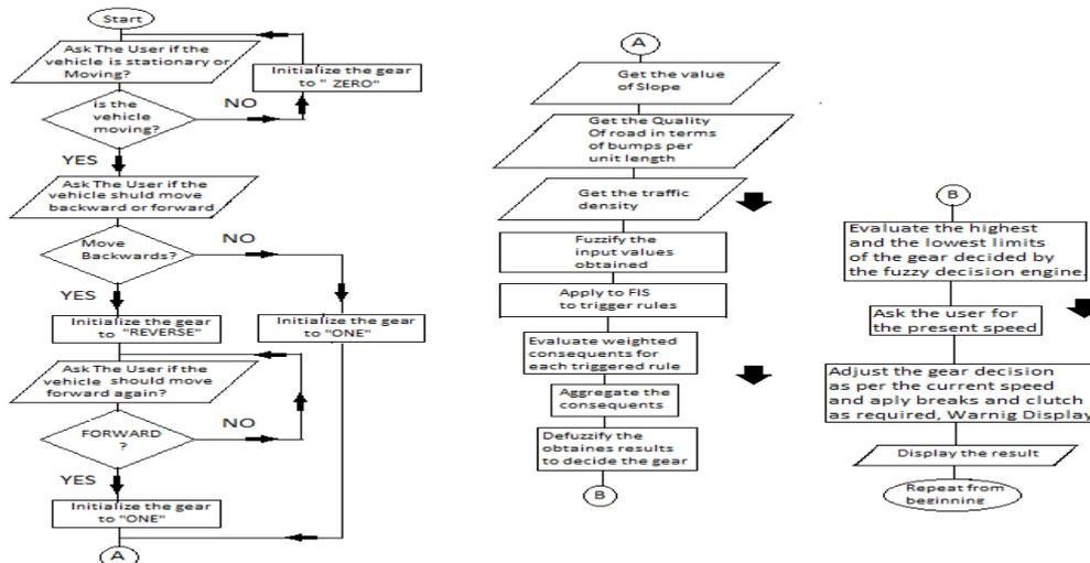
**Figure 1.** The Flowchart describing the algorithm for the FIS
