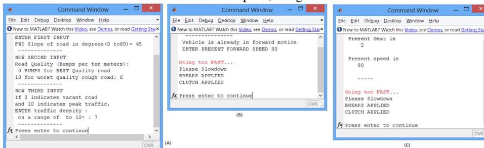
Figure 6: Vehicle is on a road condition needing First gear, but current speed is 80 KMPH. Hence the gear is stepped up to second and brakes are applied, and a warning is flashed.
