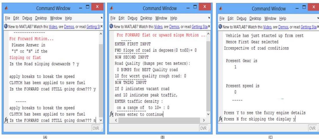
Figure 4: (A) Commanded to move forward, the system enquires about the path sloping downwards in forward direction. If so, neutral is applied. (B) For flat or upward motion forward, the system enquires about the slope, road quality and traffic condition, but regardless of the actual situations, the first gear is selected for starting from rest.
