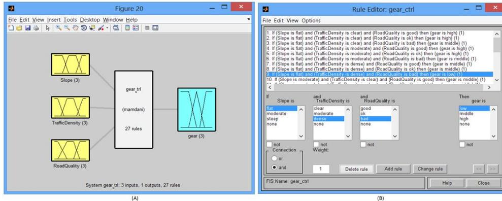
**Figure 8:** The graphical representation of (A) The fuzzy engine and (B) The ruleset.
