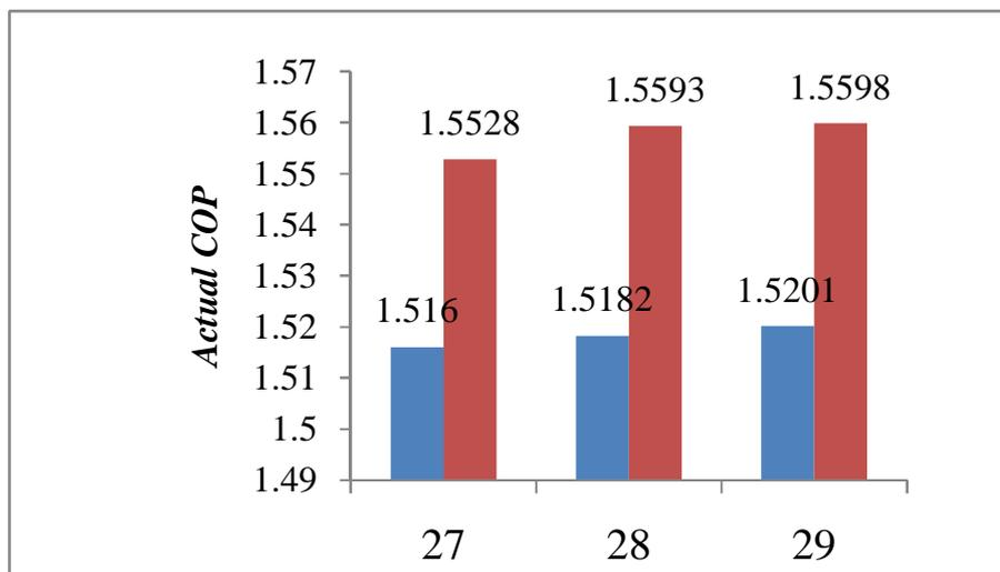
**Figure 6.** Ambient Temperature VS Actual C.O.P
