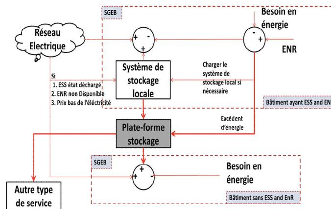
**Figure 2:** Functioning schema of the proposed platform
