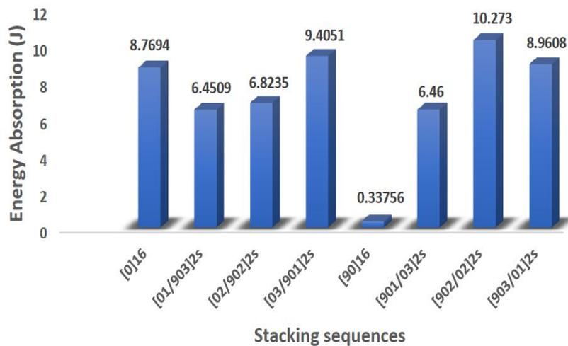
**Figure 5:** Energy Absorption of different stacking sequences of glass fiber/vinyl ester composite.
