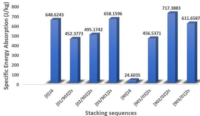
**Figure 6:** Specific Energy Absorption of different stacking sequences of glass fiber/vinyl ester composite.
