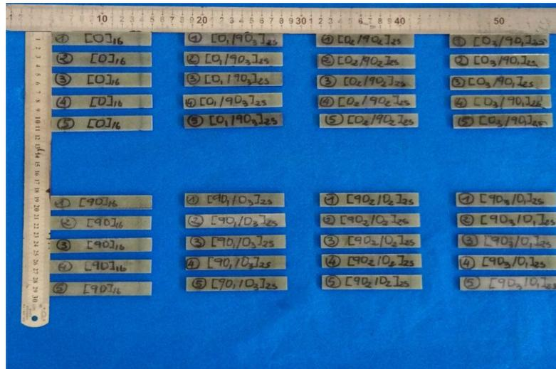
**Figure 2:** Specimens of three-point-bending test before testing.
