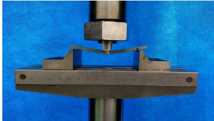
**Figure 3:** Three-point-bending experimental test of a sample.
