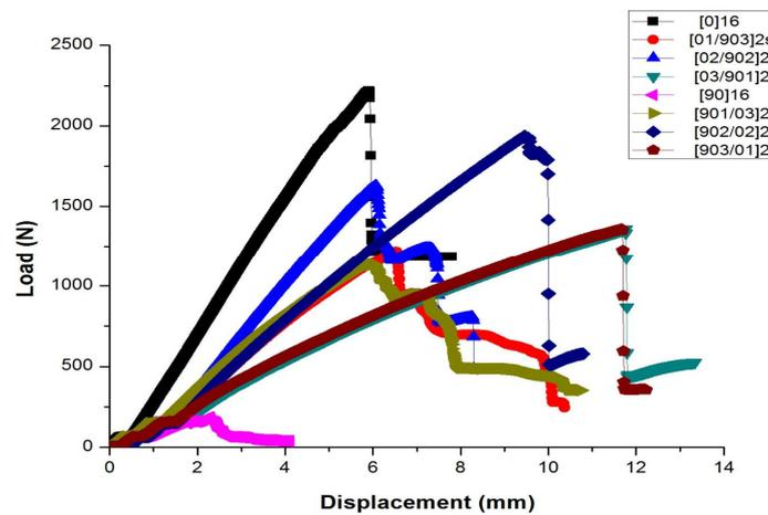
**Figure 4:** Load-displacement curves of different stacking sequences under three-point-bending test.
