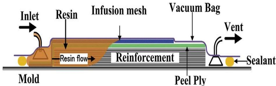
**Figure 1:** Schematic diagram of the Vacuum Assisted Resin Infusion (VARI) process [16].
