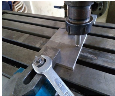
Fig 3: Conventional milling machine with work piece and tool
