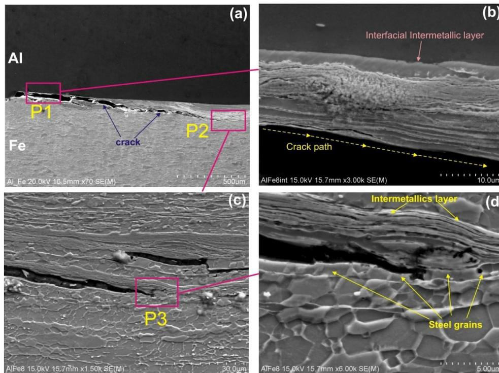
**Fig. 12** Fractured path shown in SEM micrographs of a tensile-shear sample of welds stopped at  $F_m/w_s = 265 \text{ N/mm}$  and unloaded.
