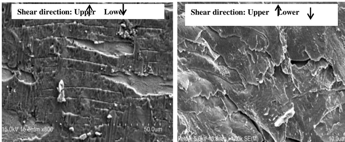
**Fig. 11** SEM Micrographs of tensile-shear tested samples in (a) Location 1 displaying heavily deformed ductile fracture of the intermetallic layer and (b) Location 2 displaying brittle fracture of the intermetallic layer
