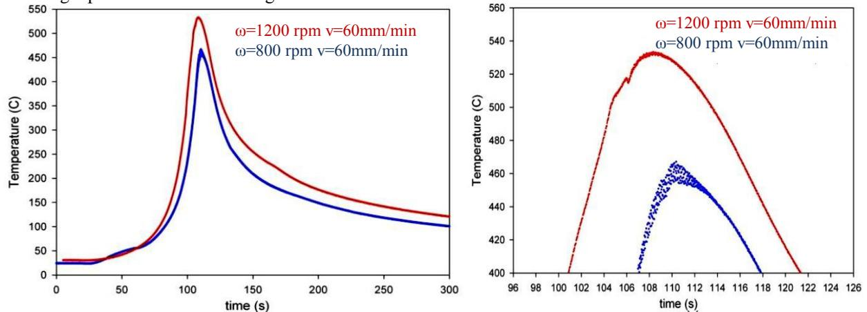
**Fig. 6** (a) Measured temperatures at the Al-steel interface region during FSLW, for the welds made using  $D_p \approx 0$  mm and  $\omega$  and  $v$  as indicated (b) enlarged view of temperature readings for temperatures  $> 400$  °C
