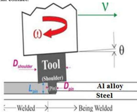
**Fig. 2** Schematic illustrations of friction stir lap welding (FSLW) of Al-to-steel with the pin having penetrated to steel
