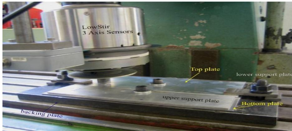
**Fig. 1** A milling machine, mounted with LowStir™ used for Al-steel FSLW experiments
