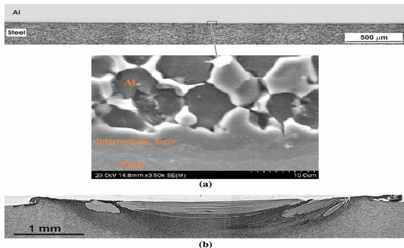
**Fig. 7** Interface microstructures of the weld made using  $\omega = 1200$  rpm  $v = 20$  mm/min (further experiment), a sample taken in Location 1—optical micrograph (top) and SEM micrograph (bottom) taken in location as indicated, b sample taken in Location 2.
