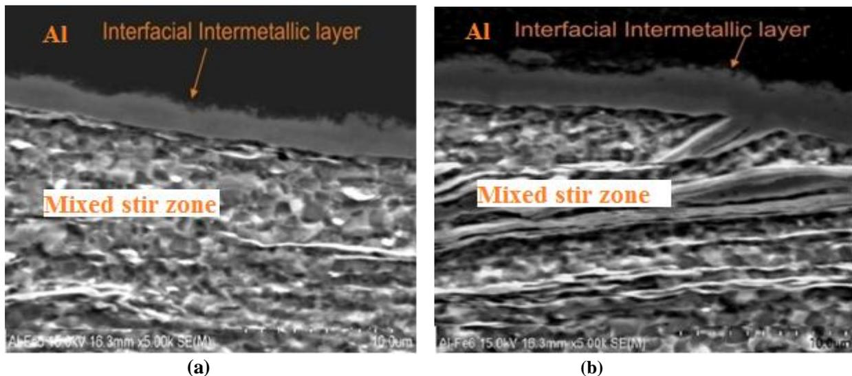
**Fig. 5** Microstructures in the interface regions of FSL welds made using  $D_p \approx 0$  mm,  $v = 60$  mm/min, (a)  $\omega = 800$  rpm and (b)  $\omega = 1200$  rpm
