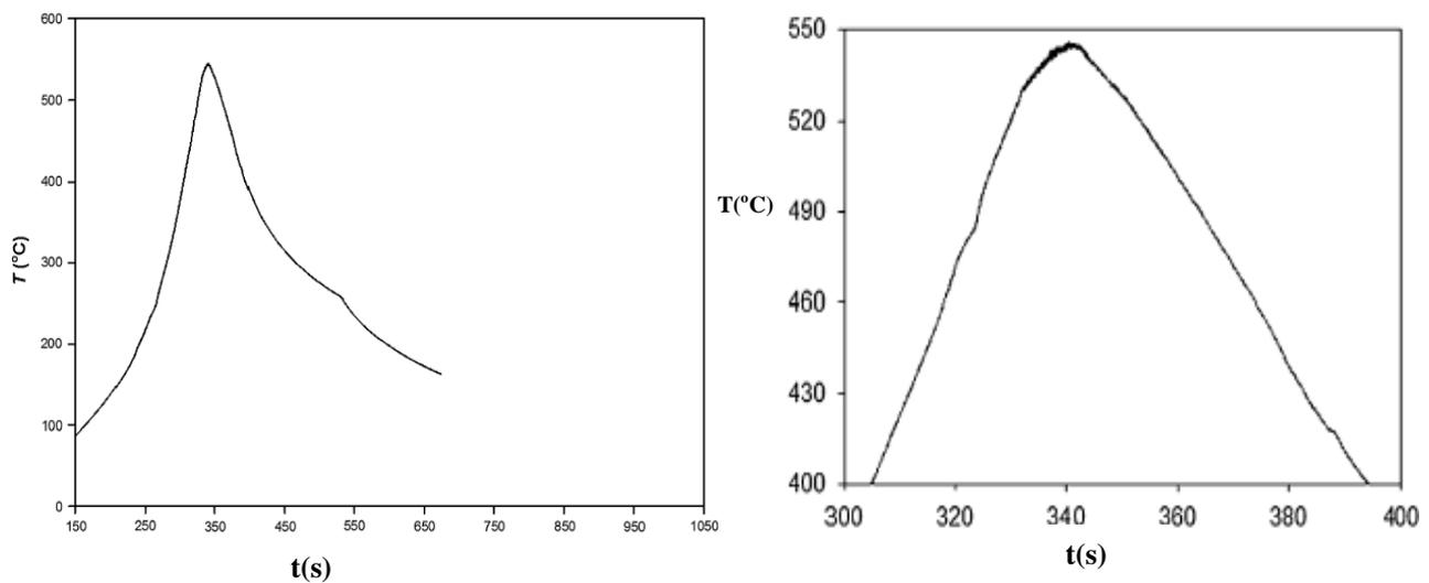
**Fig. 8** Temperature history at Al-steel interface region during FSLW for weld made in the further experiment ( $\omega = 1200$  rpm and  $v = 20$  mm/min)
