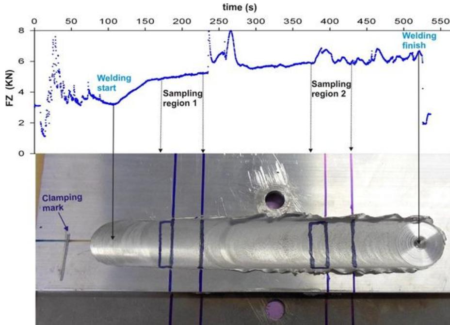
**Fig. 3** An Al-Steel FSL Weld made using  $\omega=800$  rpm and  $v=60$  mm/min with Fz – time curve, location of sampling region 1 and 2 is indicated.
