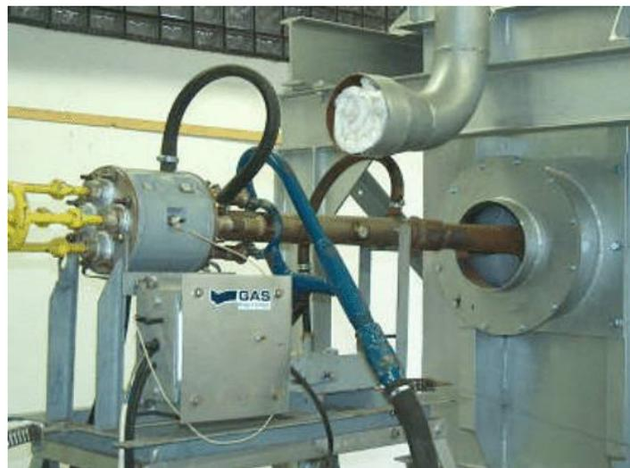
**Figure 2:** A view of the pulse combustor investigated at the MEF of University of Sarajevo
