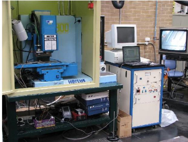
Fig:-2 The Nd:YAG laser rig with the X-Y table controller.
