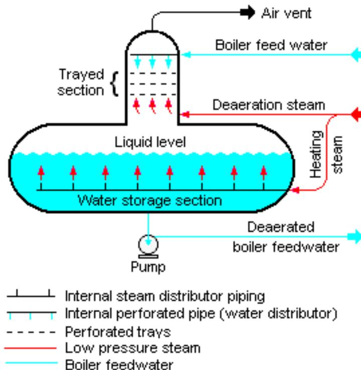
**Fig:-1** Schematic diagram of spray and tray type de-aerator
