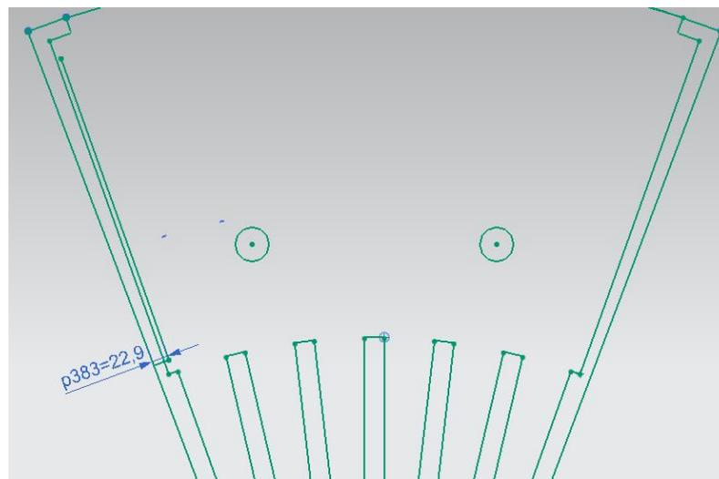
**Figure 3:** Width of the narrowest mounting position of the Gripper
