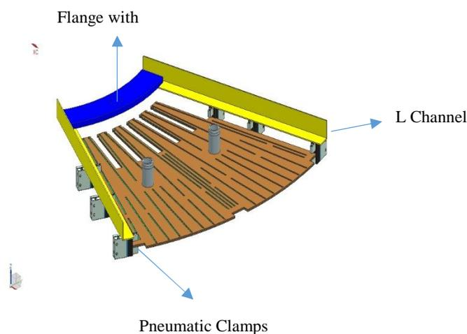
**Figure1** Design of End of Arm Tool
