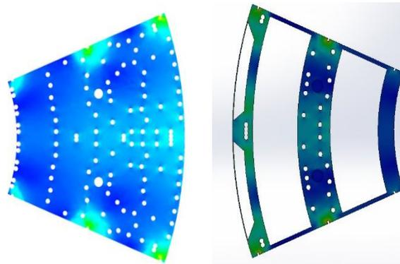
**Figure 9:** Plot of the Static Nodal Stress (von Mises stress) for the conservative (top) and optimized (bottom) design of the support plate.
