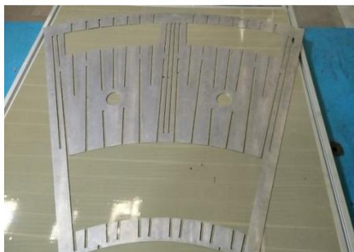
**Figure 8:** Actual Image of Guide Plate after manufacturing
