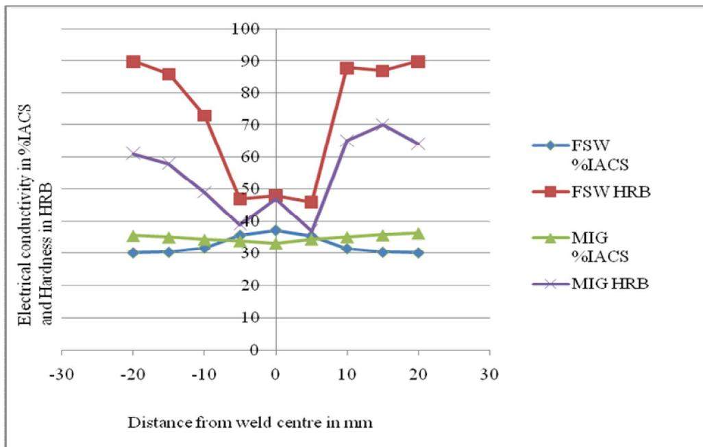
**Figure 4:** Electrical conductivity v/s hardness for FSW & MIG joints
