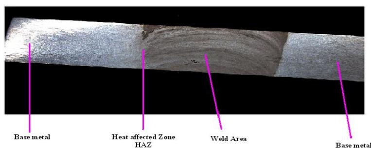
**Figure 8:** Macro graph of FSW joint
