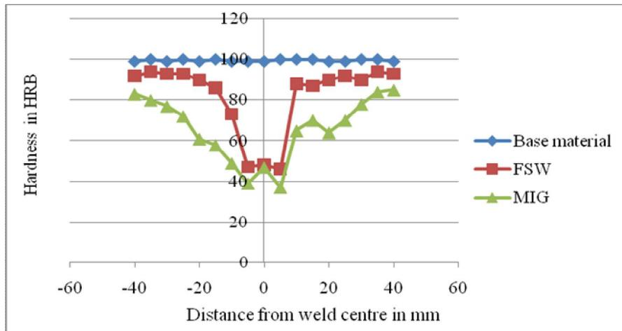
**Figure 3:** Hardness profiles for the Base metal, FSW and MIG welded joints
