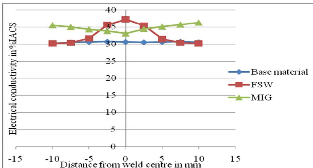
**Figure 2:** Electrical conductivity curves for the Base metal, FSW and MIG welded joints
