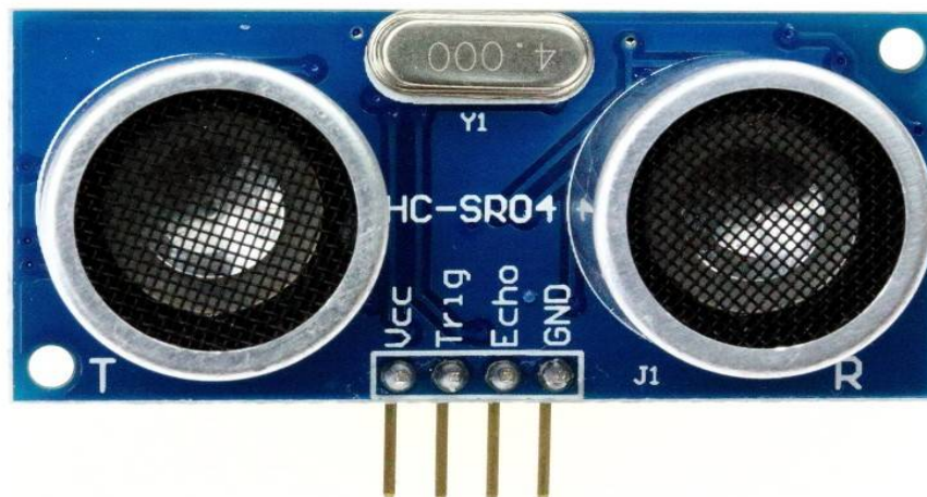
Fig:-2 Ultrasonic Sensor HC-SR04
