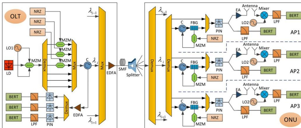
**Fig-1** UW-WDM passive optical network architecture model
