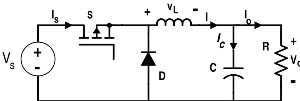
Fig:-1 Switching states and circuits of buck rectifier
