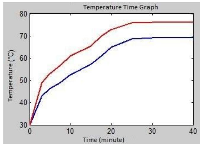
**Figure 5** Temperature-time graph of 1.5 mm<sup>2</sup> 0,3 / 0,5 kV single core low voltage cable for both load cases
