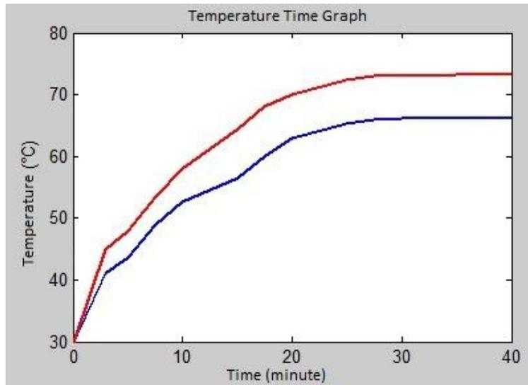
**Figure 3** Temperature-time graph of 3x2,5 mm<sup>2</sup> 0.3 / 0.5 kV low voltage multimode cable for both load cases
