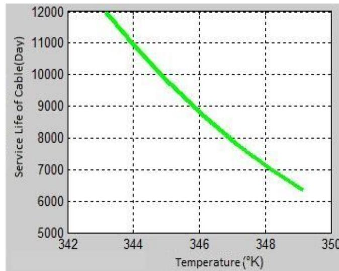
**Figure 8** Effect of temperature variation under non-linear load on the life of “3x1.5 mm<sup>2</sup> 0.3 / 0.5 kV singlecore low voltage cable”.
