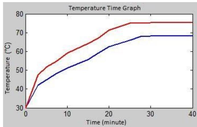
**Figure 4** Temperature-time graph of 3x1.5 mm<sup>2</sup> 0.3 / 0.5 kV low voltage multi-core cable for both load cases
