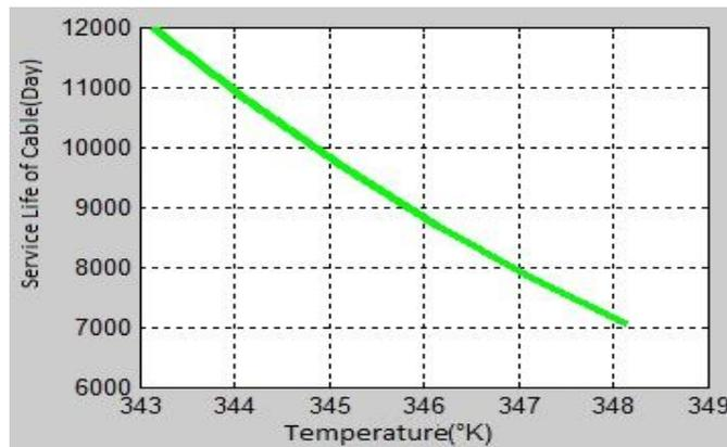
**Figure 7** Effect of temperature variation under non-linear load on the life of “3x1.5 mm<sup>2</sup> 0.3 / 0.5 kV multicore low voltage cable”.
