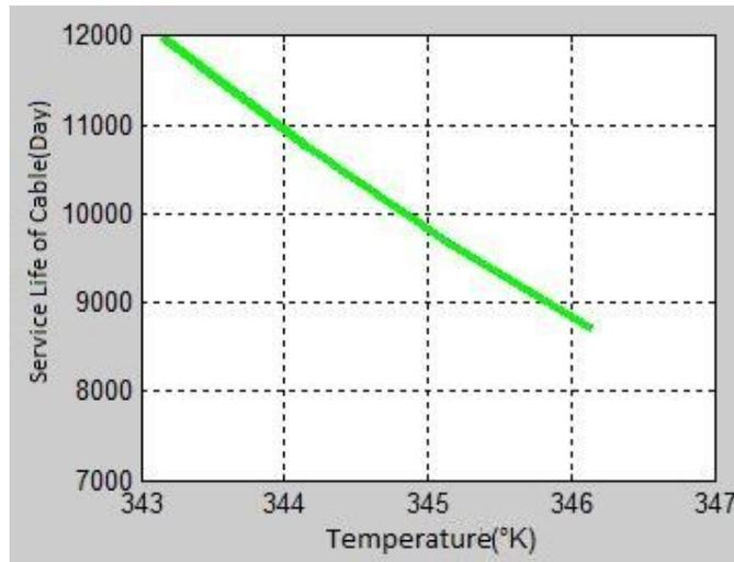
**Figure 6** Effect of temperature variation under non-linear load on the life of “3x2.5 mm<sup>2</sup> 0.3 / 0.5 kV multicore low voltage cable”.
