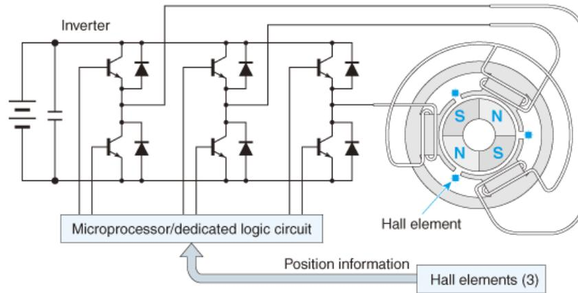
**Fig:-1** Basic Diagram of Brushless Dc Motor
