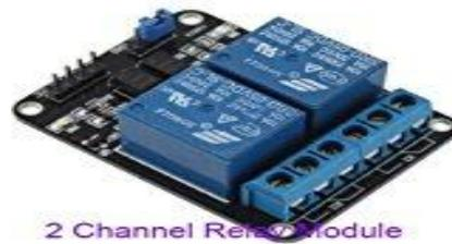
Fig. 4: Relay board
