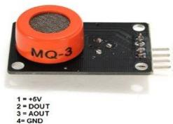
Fig.4.4. MQ-3 Alcohol sensor
