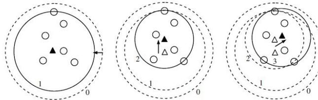
**Figure. 1.** Finding the minimum enclosing circle for six application nodes [3]. The data-node (black triangle) is placed at the center of the smallest disk that contains all application nodes (small circles).
