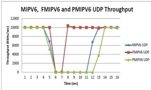
**Figure 12:** UDP passing in MIPv6, FMIPv6 and PMIPv6 between handover
