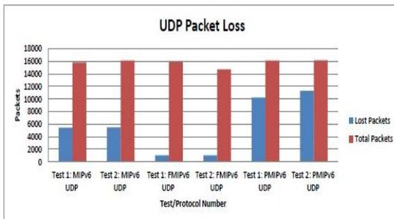
**Figure 14:** UDP Packet Loss MIPv6, FMIPv6 and PMIPv6
