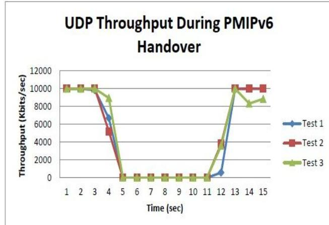
**Figure 11: UDP passing in PMIPv6 during handover**
