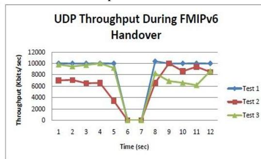
**Figure 7:** UDP Throughput in FMIPV6 during Handover
