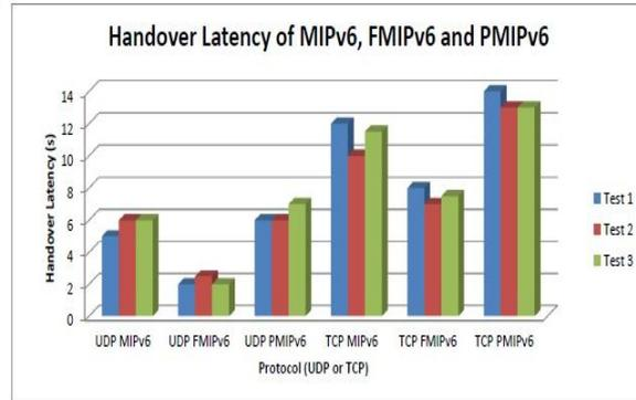
**Figure 13:** Handover Latency of MIPv6, FMIPv6 and PMIPv6
