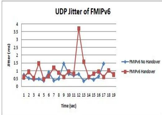
**Figure 8: UDP Jitter in FMIPv6**
