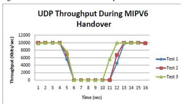
Figure 3: UDP Throughput in MIPv6 during Handover
